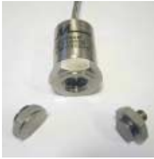
Fig 6: Transducer with Quickfit base showing adhesive and threaded adaptors
